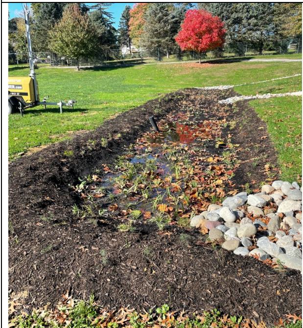
Test 1: 2"+ rain event 10/27/2021 – 24 hours after storm event ended
